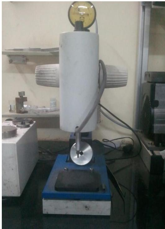
NOTE: While loading the Cutter (Rectangular and cylindrical) rotate with your hands and then with the tool mentioned in the picture rotate just about 90 degree. Please don't tight the cutters forcefully.
