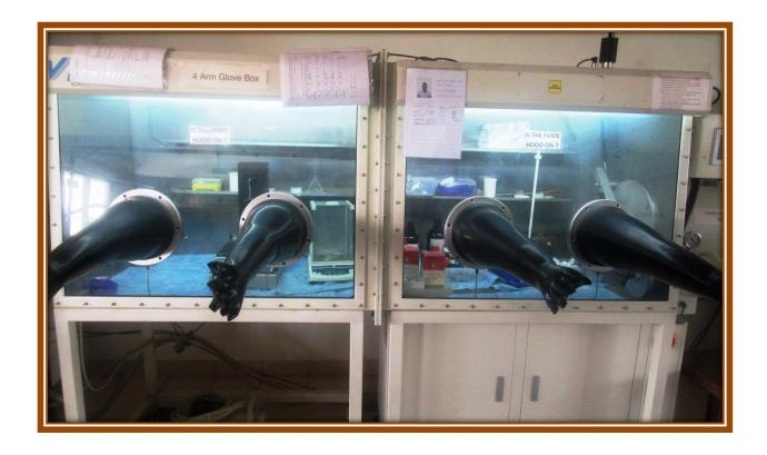
Glove box is used to store air and moisture sensitive chemicals and to do small scale processes like dip coating in inert atmosphere. While doing processes proper precaution is adopted to control rise of air and moisture level. There may be contamination issues.
