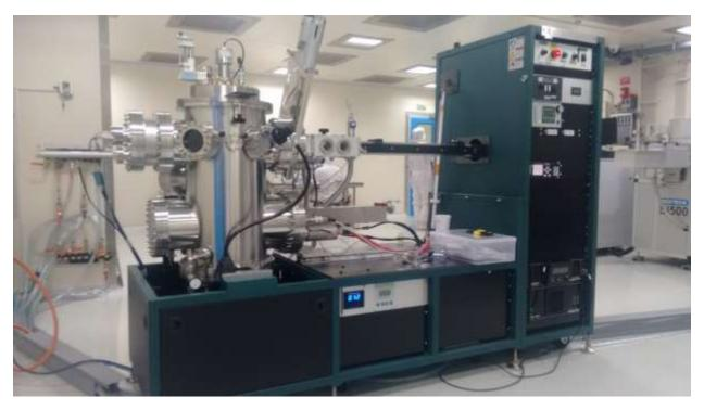
The AJA 6 target e-beam evaporator which belongs to the ATC-Orion 8E ultra high vacuum (UHV) series is a powerful e-beam evaporator with RHEED gun. It has a multi-pocket linear UHV e-beam source with slide module consisting of six 15cc crucibles with manual indexing. The system also features:-
