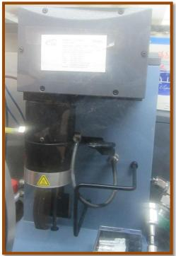
Thermogravimetric analysis uses heat to induce chemical and physical changes in materials and performs a corresponding measurement of mass change as functions of temperature or time. Thermogravimetric is performed on a wide range of materials including polymers, composites, laminates, adhesives, food, coatings, pharmaceuticals, organic materials, rubber, petroleum, chemicals, explosives and biological samples.
