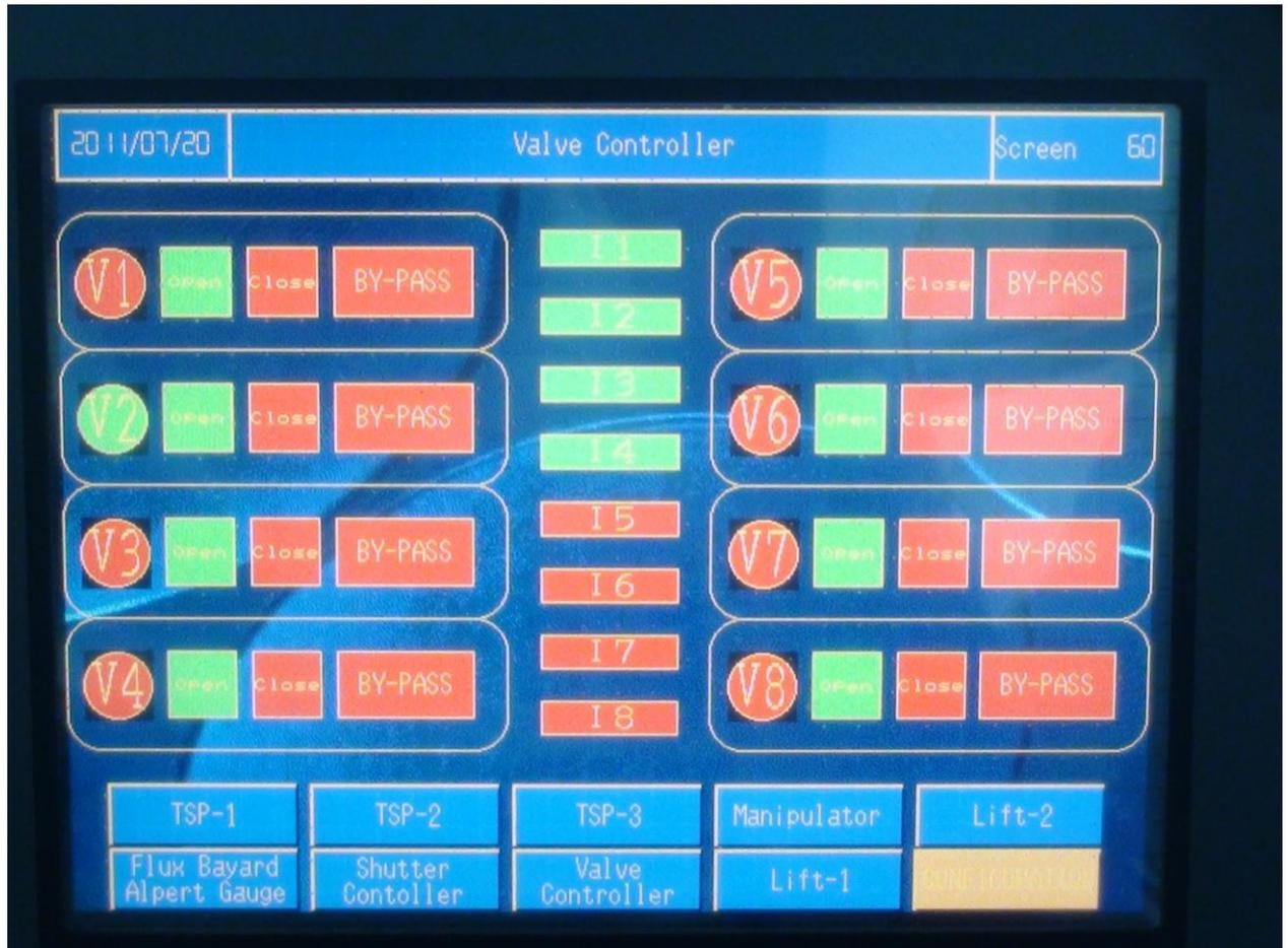
V1 valve: it is a GATE valve between cryo pump and growth chamber.
