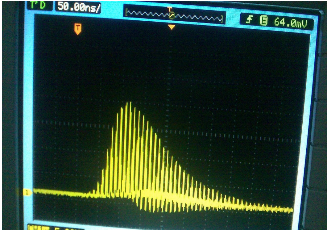
Fig: 5 Picture showing Mode-locked beam on the CRO display.
