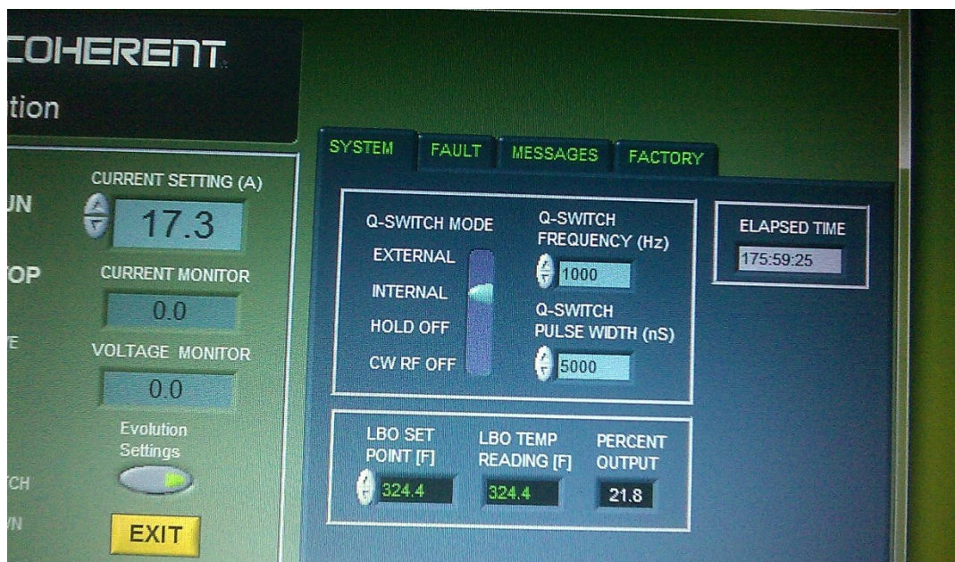
Fig 3: Picture showing front panel of the Evolution software indicating the current, Voltage & System settings.
