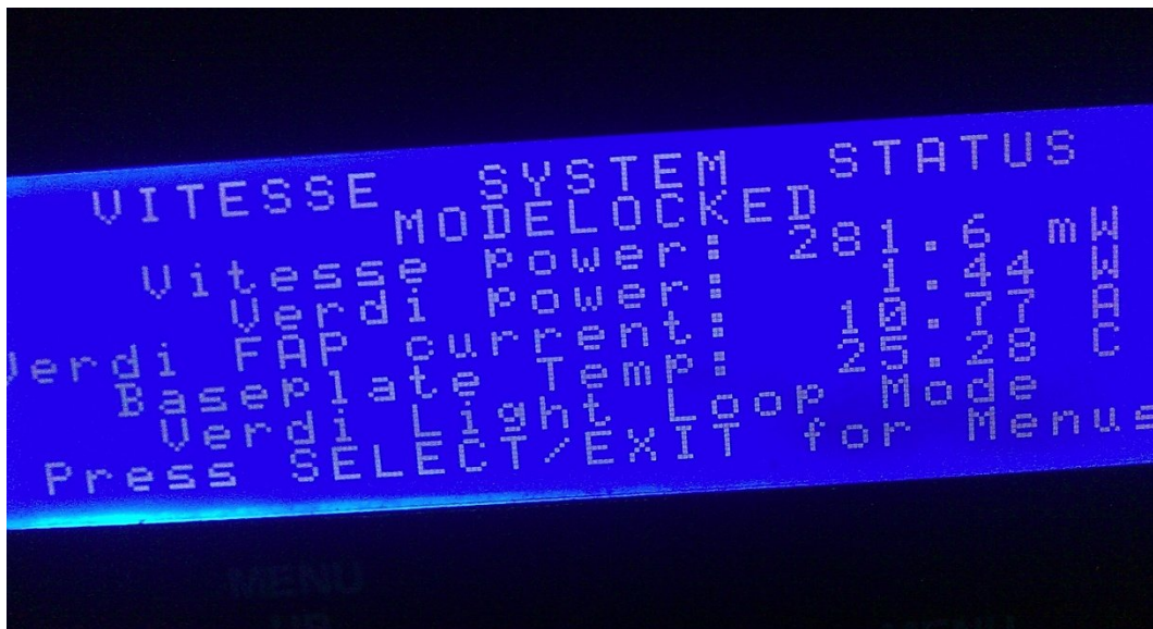
Fig 1: Picture showing front panel of the VITESSE (as Vitesse system status) indicating Mode-Locked condition
