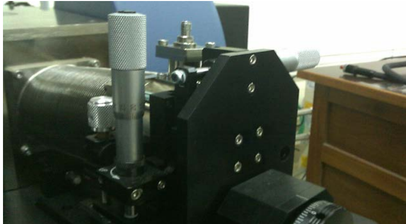
Fig. Z-direction movement caliper (Up and down movement of probe)
