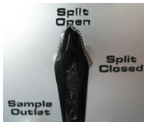
Figure 14 How to change the split flow
