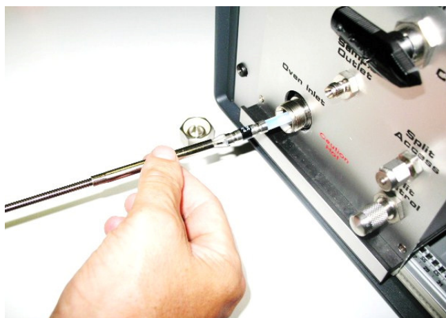
Figure 9 – Always use the supplied extraction tool
